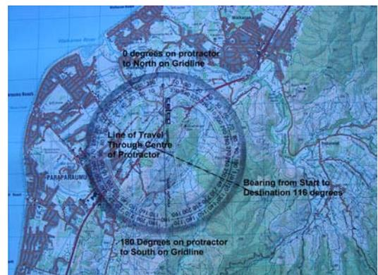
4. Orient the protractor so that the 0 mark is directly above (to the north of) the start. That is, the line between the centre of the protractor and the 0 mark should be parallel with the vertical grid lines on the map.
